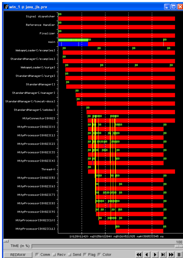
Figure 7. Paraver visualization of a SURGE generated workload over Tomcat v4.0
