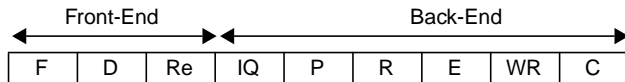
Fig. 1. Processor Pipeline. F: Fetch, D: Decode, Re: Rename, IQ: Issue Queue, P: Read Payload, R: Read Register File, E: Execution; WR: Write Register File, C: Commit.
