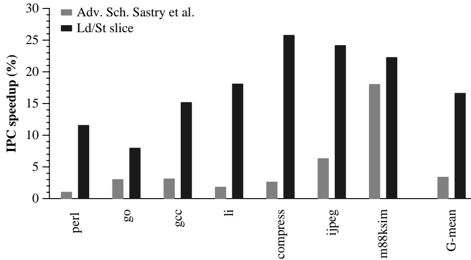
Figure 3-3: Static versus dynamic LdSt slice steering
