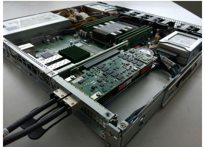
Fig. 2 Active network probe implemented in a small factor server. FPGA is placed in the bottom corner, with both QSFP28 interfaces connected. Management interfaces are on the left.
