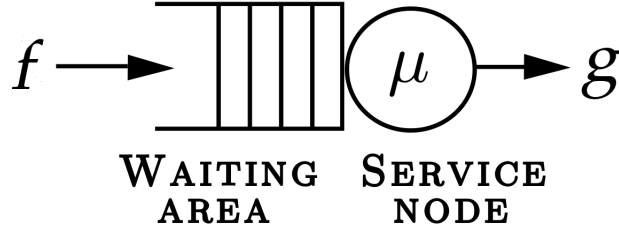
FIGURE 1. Example of a system with a queue and a server of speed \mu .
