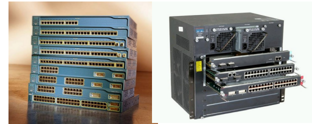
Edge and backbone CISCO switches.
